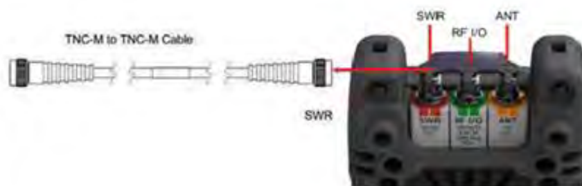
Figure 18: VSWR Calibration Setup Diagram
