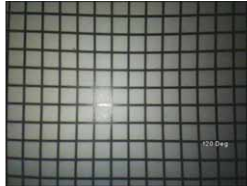
120° optical tip, distortion correction on
