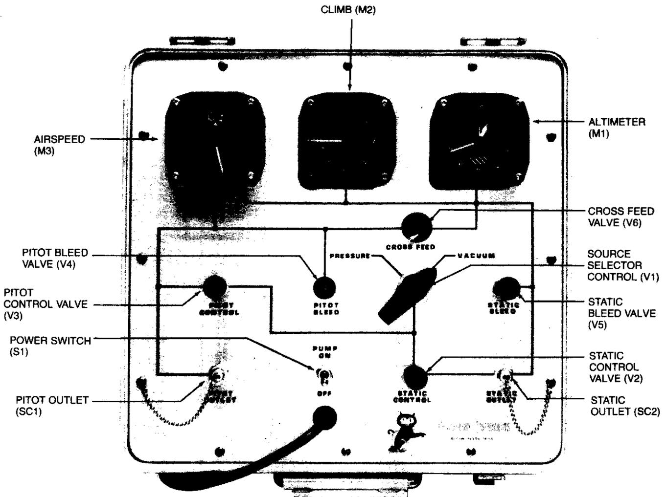
Figure 4.1 377-4 Pitot and Static System Tester, Control Panel
