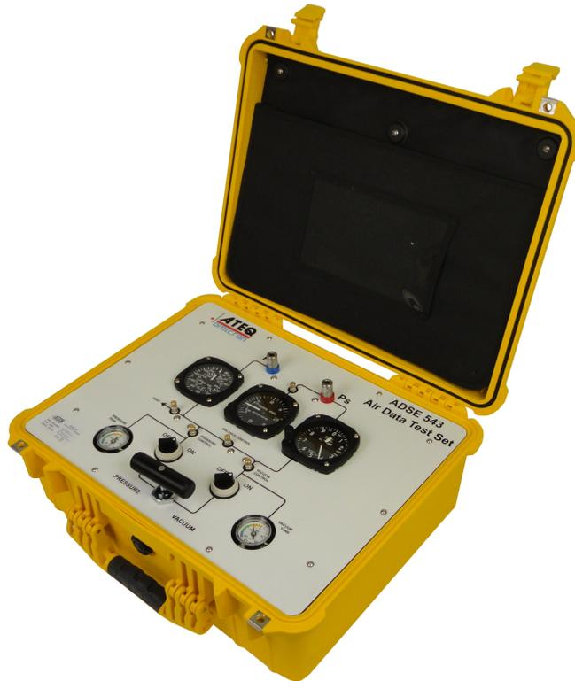
The ADSE 543 pitot static tester, housed in a plastic carrying case, is a portable, self contained field tester designed to test aircraft pitot and static systems for leaks as well as the operation and calibration of airspeed, altimeter, engine pressure ratio, manifold pressure indicators, and other vacuum or low pressure units.
