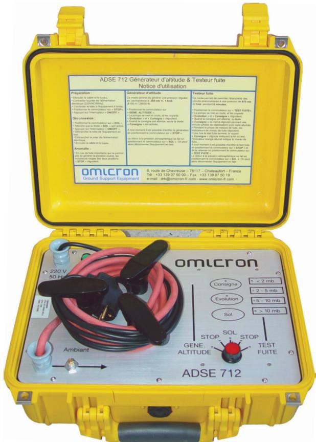
The ADSE 712 is a single channel generator that simulates an altitude to test different pneumatic equipments for aerospace applications or equipment reacting to barometric constraints.
