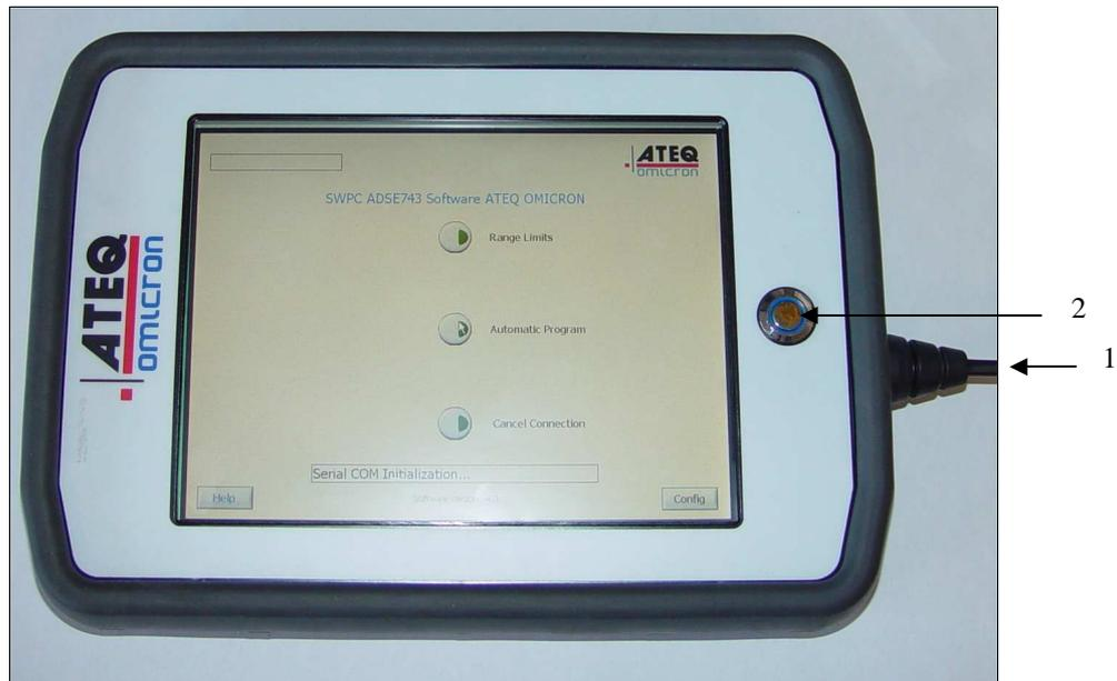
*Figure 1: ADSE743 remote control front panel*
