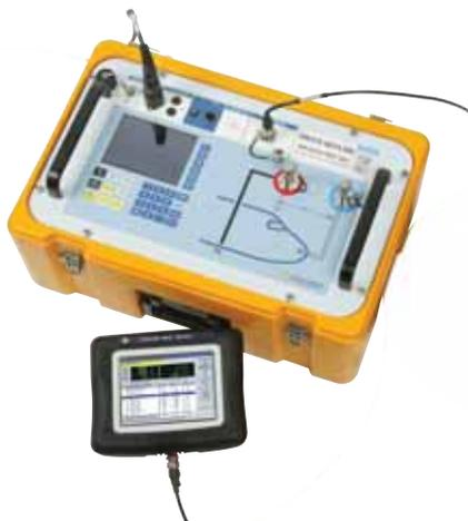
The ADTS 505 option (B) Advanced Hand Terminal significantly enhances operation of the Druck ADTS 505 Air Data Test Set. Specifically designed to meet the safety on the flightline regulations. The advanced hand terminal enables a single operator to implement sophisticated test routines whilst seated in the aircraft cockpit. Aircraft testing time and the possibility of communication errors are therefore both reduced.
