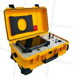
Case meets required measurements to fit into overhead compartment in commercial airlines. Exterior case dimensions: 22"L x 14"W x 9"H, 55.1cm L x 35.6cm W x 22.9cm H. Weight 37 lbs., 16.78 kgs.
