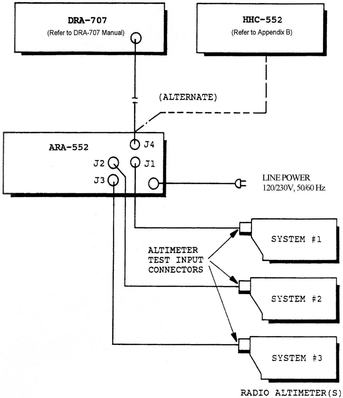
Figure 4-1 - Basic Equipment Set-up
