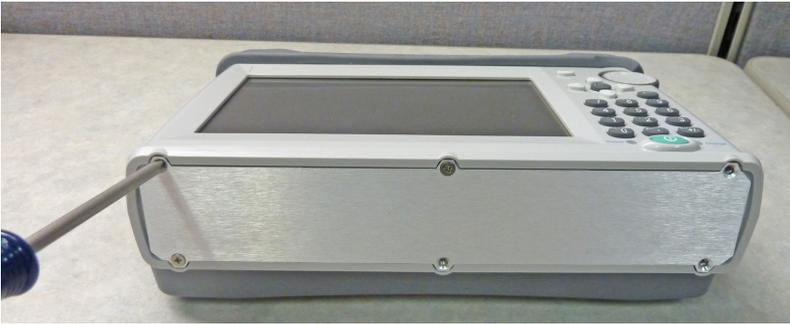
**Figure 10-2.** Remove the Battery Cover Plate
