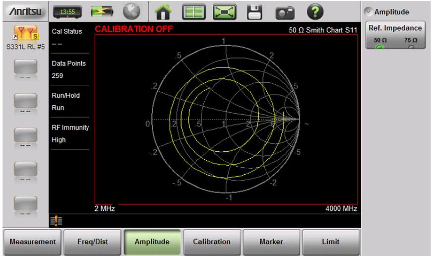
Figure 3-20. Set Reference Impedance for Smith Chart Calculations
