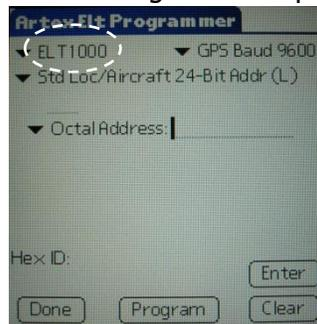
**Figure 11: ELT 1000 Will Display Baud Rates**
