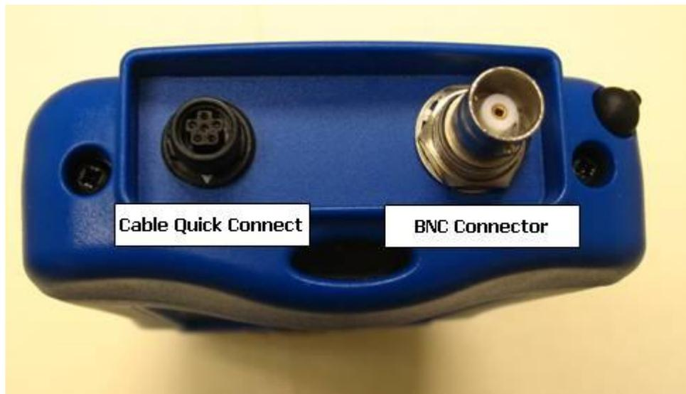
**Figure 2: Handheld Programmer Connectors**
