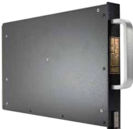
AvtechTye's CTS-700 Ramp Tester tests Avtech's ARINC 714 standard SELCAL decoders without any additional equipment directly on the aircraft without the need for ground radio facilities
