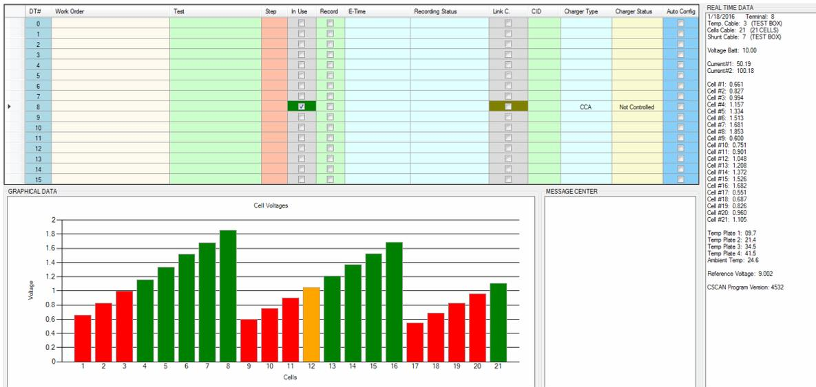
Figure 76 - Cells simulation for one 21 cell battery
