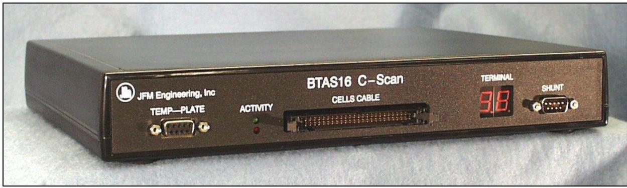
**Figure 10 - C-Scan Front Panel**
