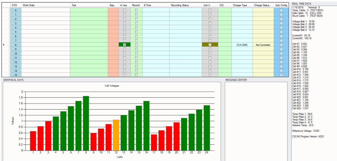
Figure 73 - Cells simulation for a 24 Cells
