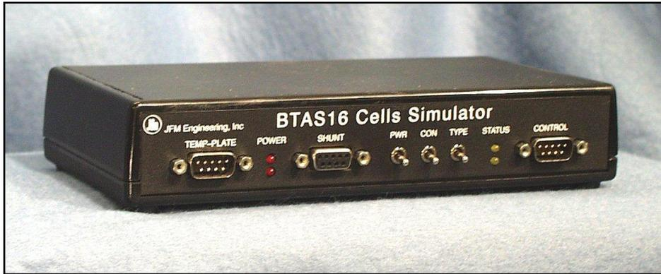
**Figure 78 - Cell Simulator Front Panel Switches**
