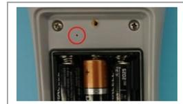
Figure 7: Alignment Access Hole Location
