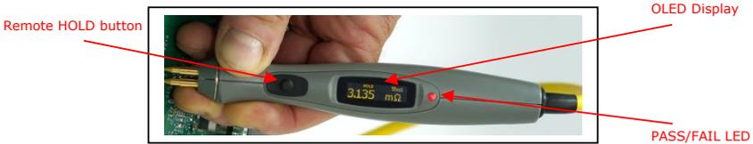
*Figure 6: Display Probe Controls*
