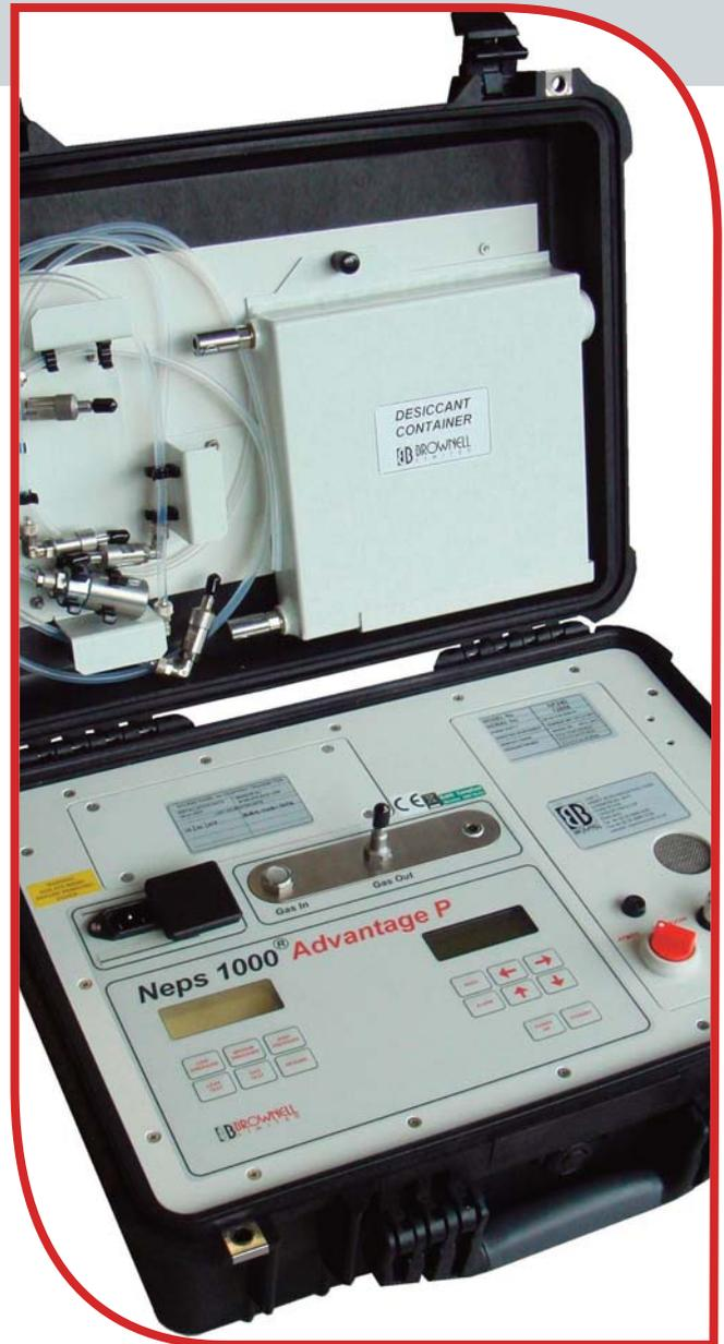
The moisture adsorber can be readily exchanged when it is saturated and requires replacement. The NEPS1000 DUAL VOLTAGE contains one Kilo of moisture adsorbing molecular sieves which are capable of adsorbing more than 20% of its own weight in moisture vapour before it is saturated. The NEPS1000 DUAL VOLTAGE is ideally suited if bottled dry gas is not available or cannot be handled or transported to the point of use.
