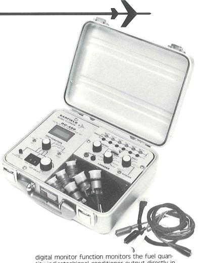
tity indicator/signal conditioner output directly in pounds, volts, ratio, etc., depending on the module.
