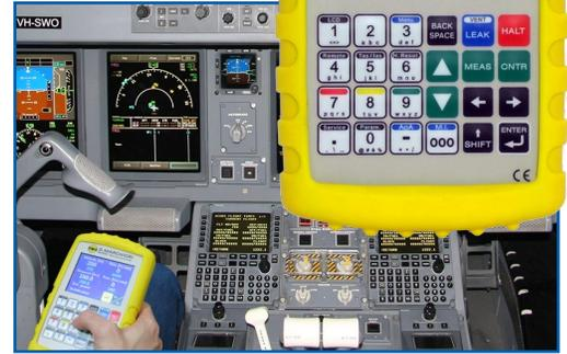
Optional multiple line switching. Up to 8 Static lines and 4 Pitot lines
