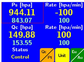
All the important air data functions are simultaneously displayed on all interfaces, constant screen or menu changes are not required. Readings of both commanded and measured test values are displayed.
