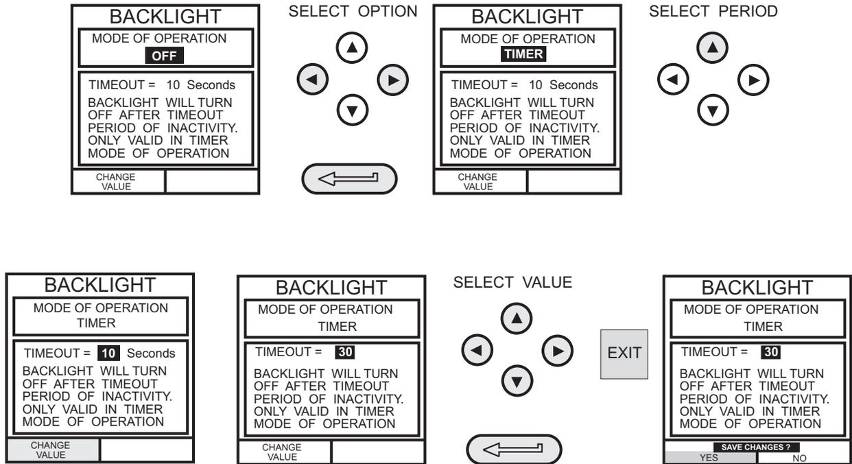
If **TIMER** mode is selected, any key press switches on the backlight for the **TIMER** period.
