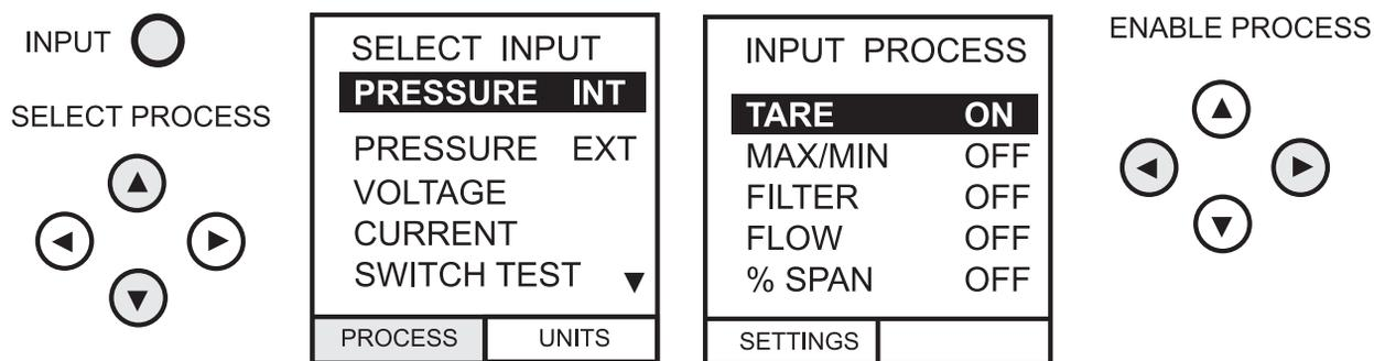
Press **ENTER** to switch the process ON with existing settings or F1 to change process settings (where applicable).
