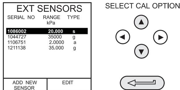
If the sensor to be calibrated is not in the directory, or no sensors are listed in the directory, press the **F1** key (ADD NEW SENSOR). This will place the sensor in the directory, allowing it to then be selected.
