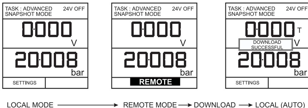
After the procedure file has been downloaded, the instrument is usually returned to the LOCAL mode by the last command in the procedure file. If the instrument remains in REMOTE mode, switch it OFF and ON to reset it.
