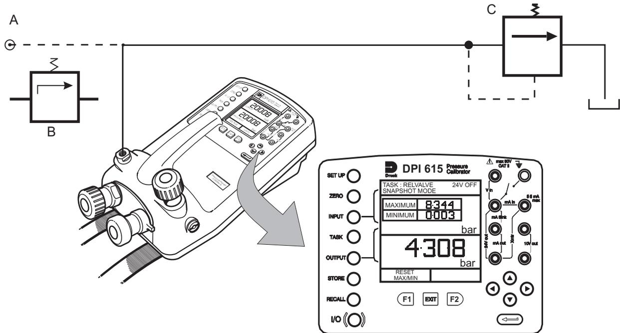
A - External pressure source (indicator instruments only)    B - Pressure regulator
