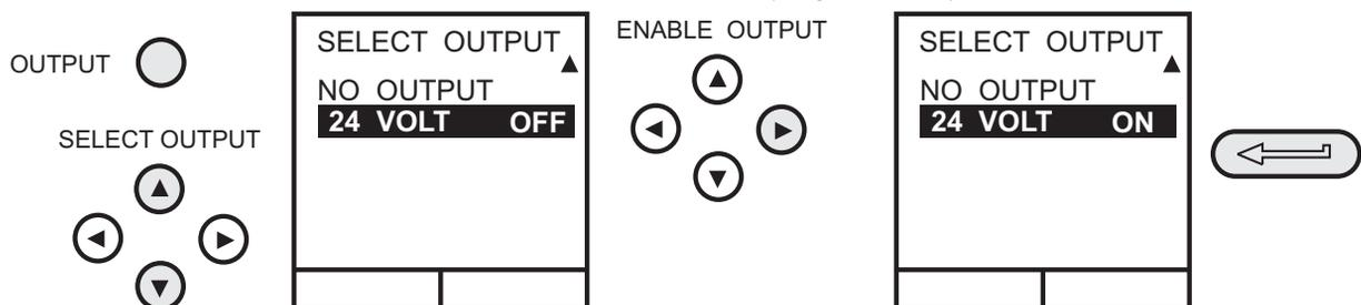
**Note:** To conserve battery power, keep the 24V supply switched off when not in use (even if the output is unloaded).
