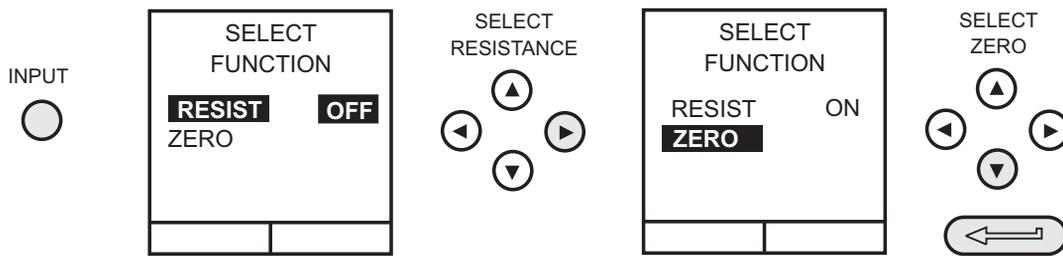
To ensure accurate measurements it is recommended that the zero procedure (that compensates for the resistance of the test leads) is carried out before performing this test.
