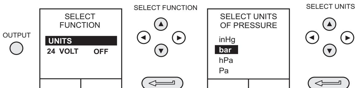
**Note:** If the four units displayed are not the units required, press **SETUP**, select **SETTINGS** and refer to page 38.
