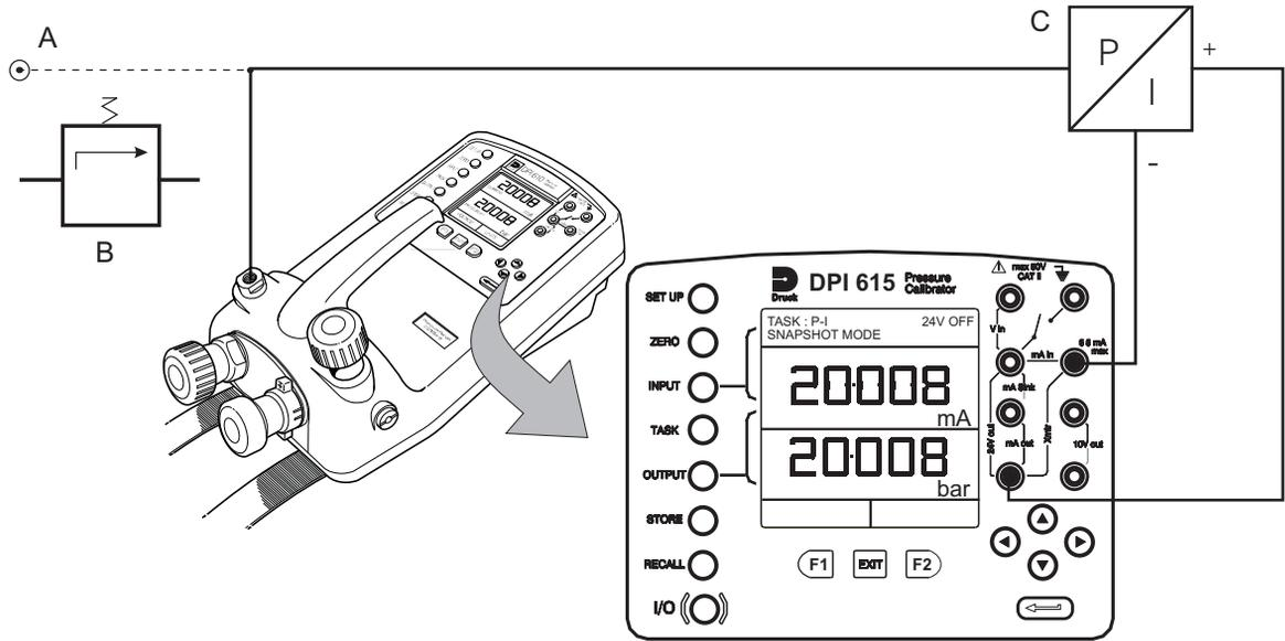
A - External pressure source (indicator instruments only)      B - Pressure regulator
