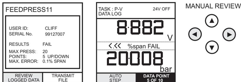
To transmit the selected logged data via the RS232 interface, connect the instrument to a free port on an external PC, ensure that the instrument's RS232 parameters match those of the PC.
