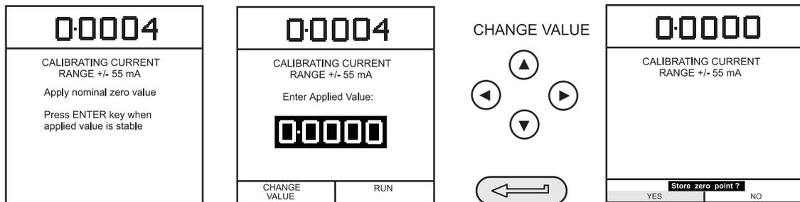
(4) Connect the mA in terminals of the instrument to a variable current source and connect a digital milliammeter in series with the supply:
