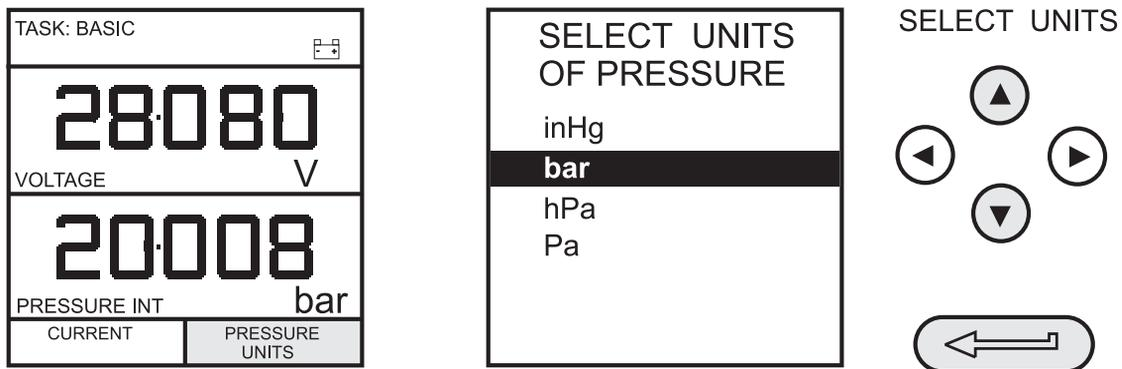
In **BASIC** mode, the instrument is configured to carry out basic Pressure to Voltage (**P to V**) or Pressure to Current (**P to I**) tests, a typical test procedure follows.
