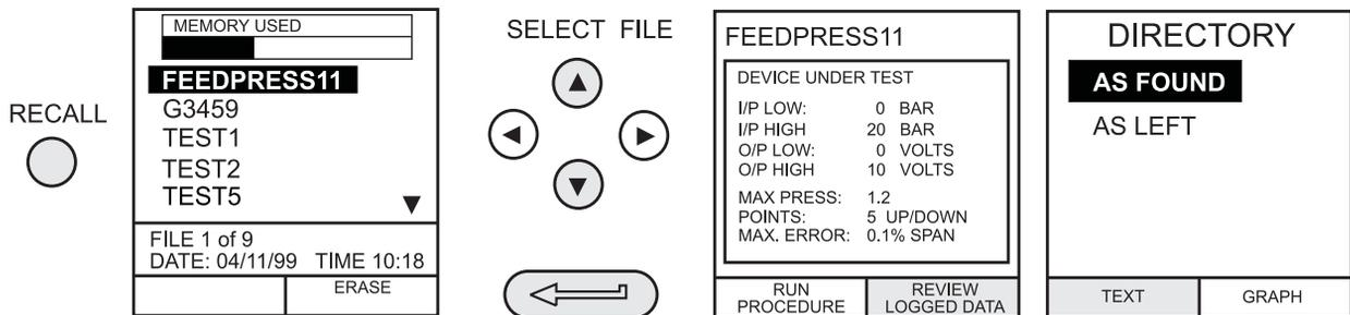
Use the cursor keys to select either the AS FOUND option or the AS LEFT option for display. AS FOUND is the result of the first run of a procedure and AS LEFT is the result of the last time the procedure was run.
