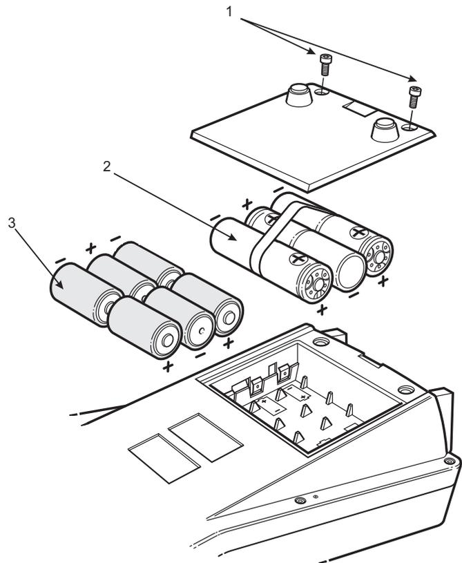
**Caution:** Old batteries can leak and cause corrosion. Never leave discharged batteries in the instrument.
