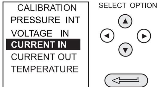
(3) Open circuit the **mA in** terminals and enter the zero point:
