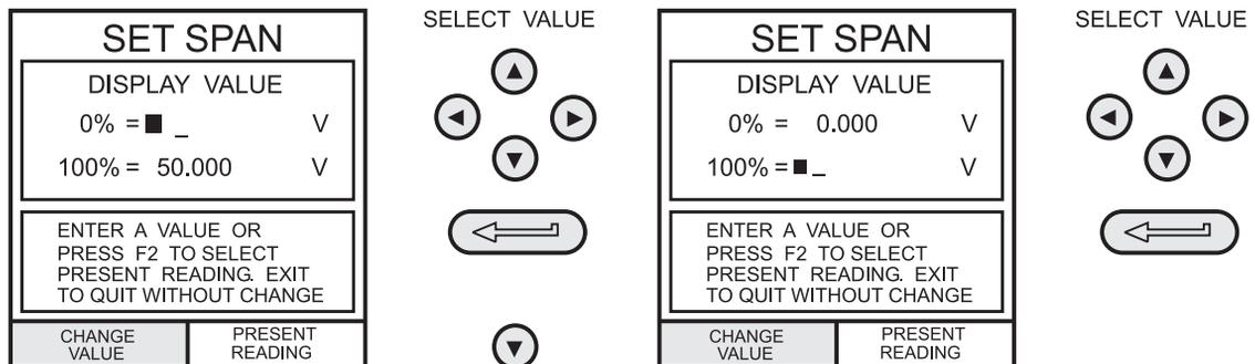
To cancel **%SPAN**, press **INPUT** and turn function **OFF** at the process menu.
