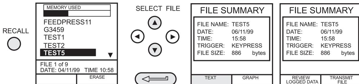
Data Log files can be displayed either as text (stored screens) or in graphical form. To display as text, proceed as follows from the File Summary menu. Select Auto Step to automatically review each screen at 1 second intervals or use the **left** ◀ or **right** ▶ cursor keys to manually review.
