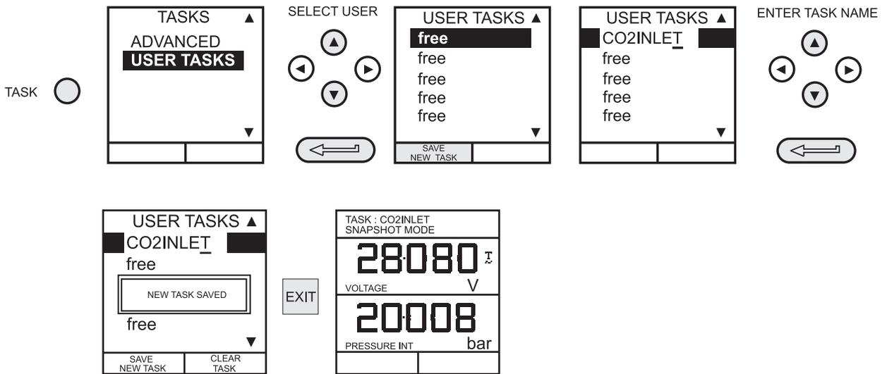
On completion of this procedure, the display reverts to newly set-up task as shown:
