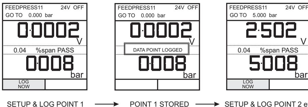
When the test procedure for a given UUT has been completed, the result of running the first test is stored as an AS FOUND file. This file cannot be overwritten. Any subsequent tests on the device are stored as an AS LEFT file that is overwritten each time the procedure on this device is run.
