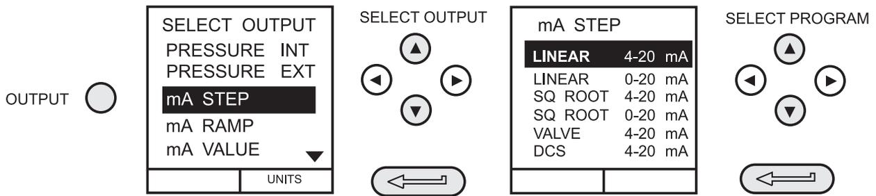
On selection of (e.g.) Linear, the output display window changes to show the selected program of output currents:
