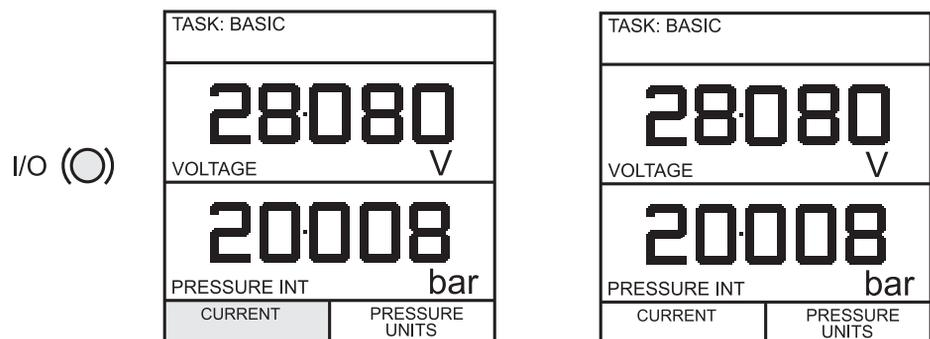
The first time the instrument powers up, it will be in **BASIC** mode with the main screen displaying voltage in the input display area and pressure in the output display area. To switch to **CURRENT** as input, press **F1** as shown. Similarly, **F1** to return to **VOLTAGE**.
