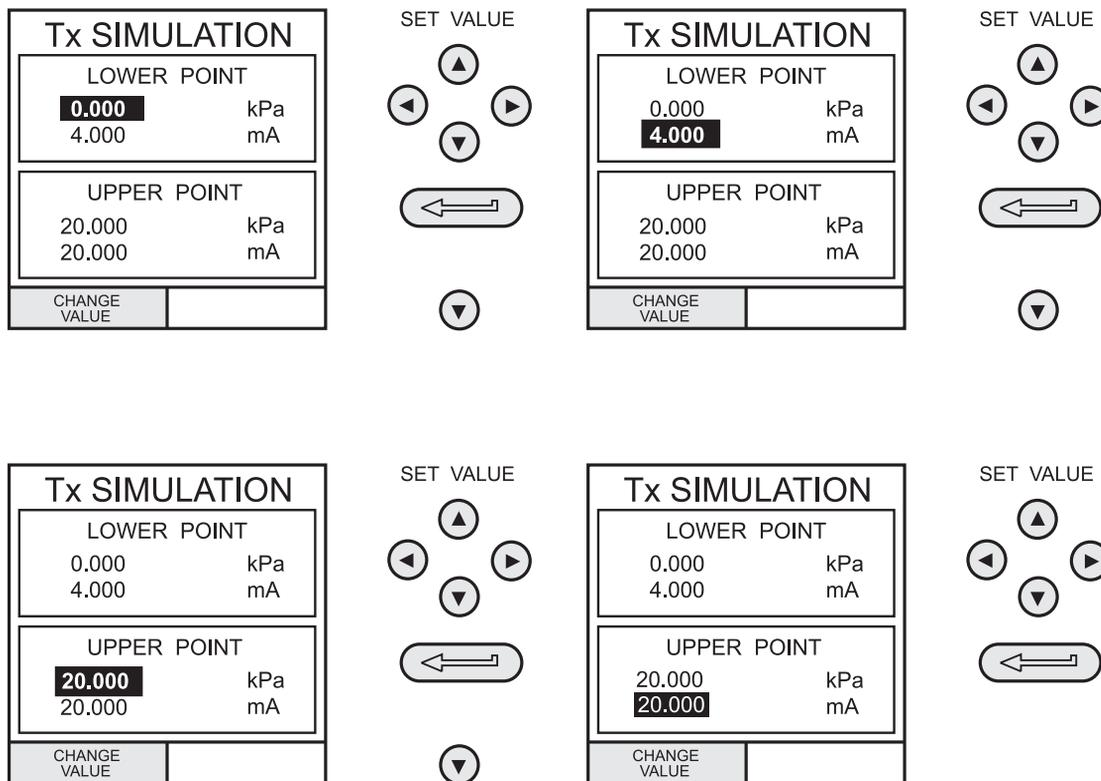
On completion of **TX SIM** set-up, the display is configured as follows:
