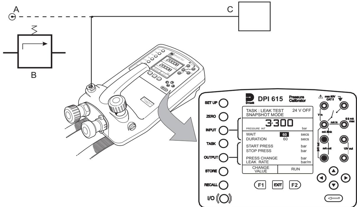
A - External pressure source (indicator instruments only)      B - Pressure regulator
