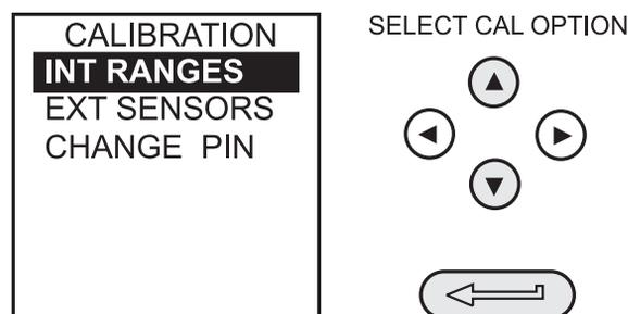
Select the **INT RANGES** from the menu as shown above and follow the calibration procedure on the display.
