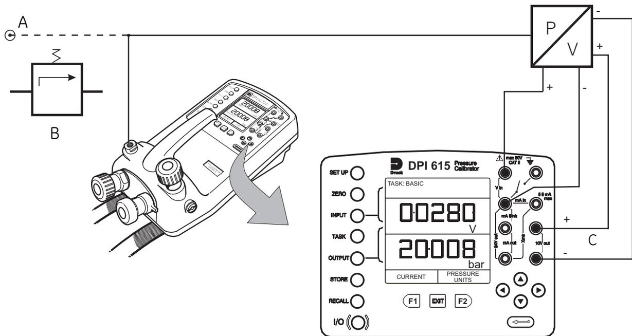
A - External pressure source (indicator instruments only)    B - Pressure regulator
