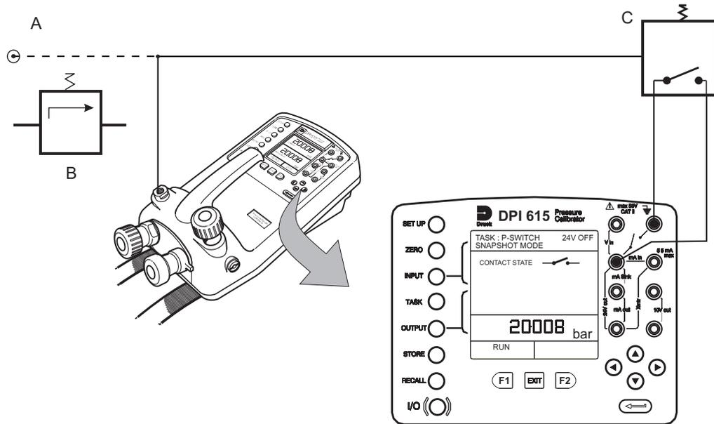
A - External pressure source (indicator instruments only) B - Pressure regulator
