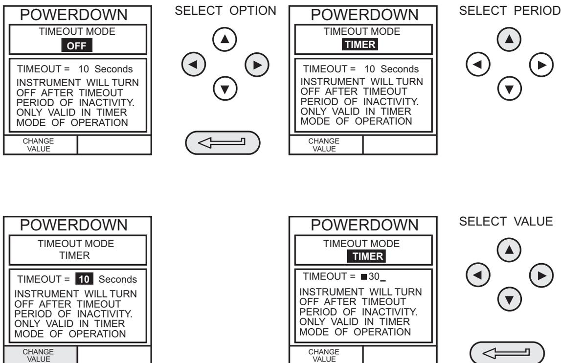
If selected to **TIMER** mode, following a period of inactivity, the instrument automatically powers off after the preset **TIMER** period.
