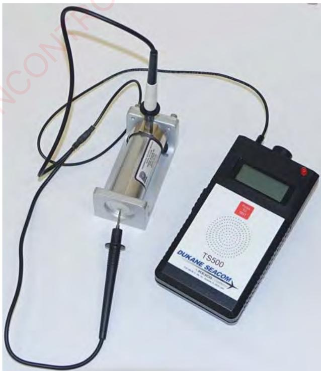
*Figure 2. Testing Beacon*
