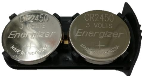
Figure 12. Batteries are placed with positive side up.
