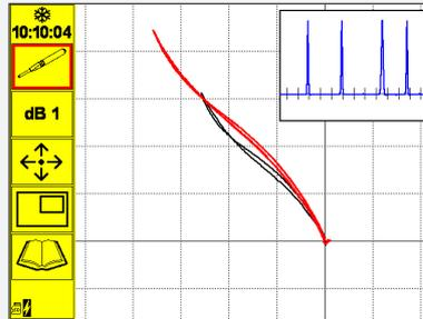
**TRACE FEATURE:** The trace function allows a reference waveform to be stored on the screen and appears along with the live spot. This allows the operator to readily compare the live data with the reference calibration.
