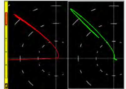
**AUTO-MIX FEATURE:** A dual frequency mix exploits the phase and sensitivity change between two different types of indication to suppress one and enhance the other.
