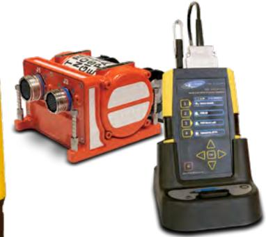
The Handheld Multipurpose Interface (HHMPI) is a portable shock-resistant tool designed to download data from Flight Data Recorders (FDR) and audio from Cockpit Voice Recorders (CVR). The HHMPI is connected to the recorder via a recorder-specific interface cable which identifies the attached recorder type.
