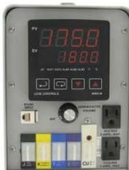
Function: Closed-loop PID controller of Heat Gun or Heat Blanket
