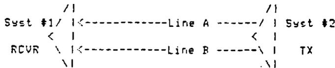
While no restriction is placed on the bus length or on the number of receivers on a bus, it is recommended that no more than 20 receivers are connected to a transmitter port in a aircraft the size of a B-747 or smaller. See figure.
