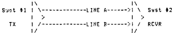
If two way communications is required then a second bus using another Tx-Rx port is required. See figure.
