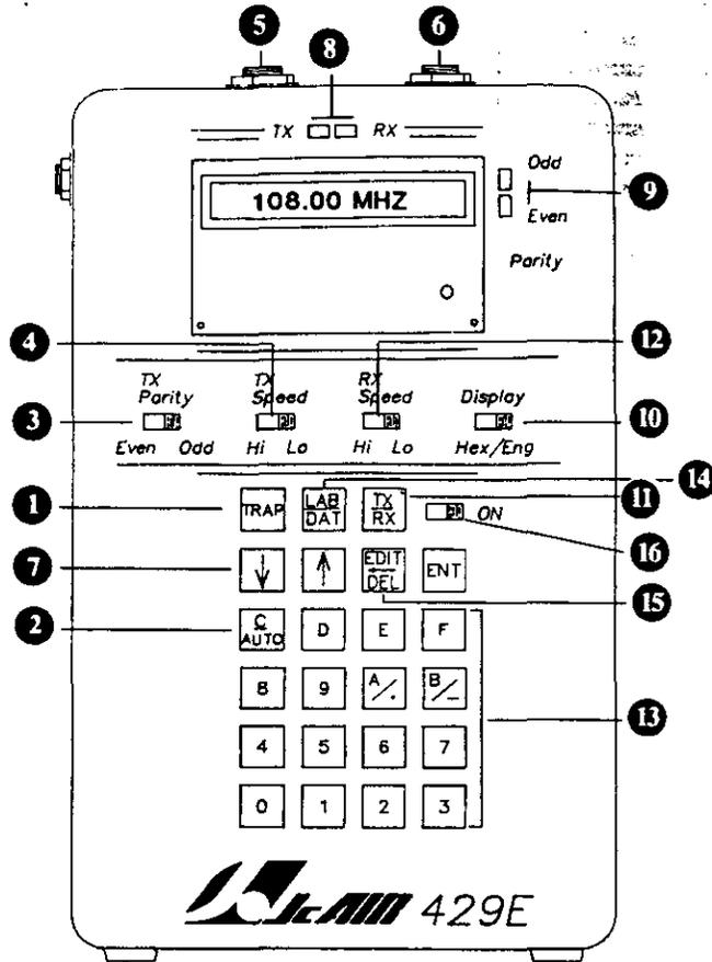
13 **Data entry keys** - allows operator to enter transmitted data in hexadecimal or engineering formats.
