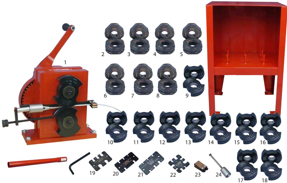
Table II-1 - Type II Bench Swaging Tool Kit - Loos Part No. M2-K
