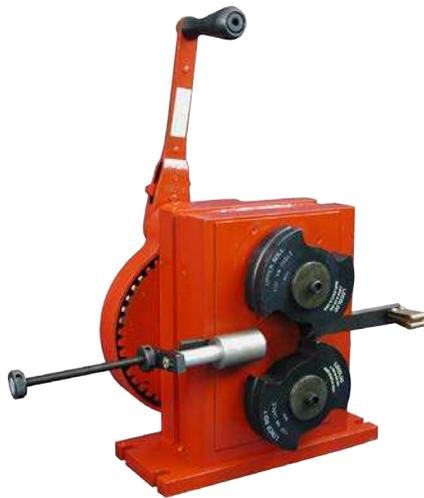
**Figure II-8** Feed Guide Assembly installed in Machine
