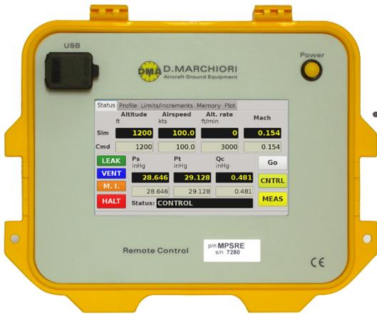
Optional MPSRE2 Multi-colored backlit 7" LCD touch screen hand terminal
