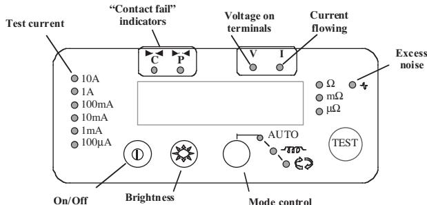
Press the On/Off switch to turn DLRO 10 on. All lamps will light, V and I lamps will flash, the software version will be displayed and the  $\Omega$  lamp will light. If the test leads have not been connected to the test sample the 'C' and 'P' lamps will also light. Press the On/Off button again to turn the instrument off. If the instrument is not used for 5 minutes it will be turned off automatically.
