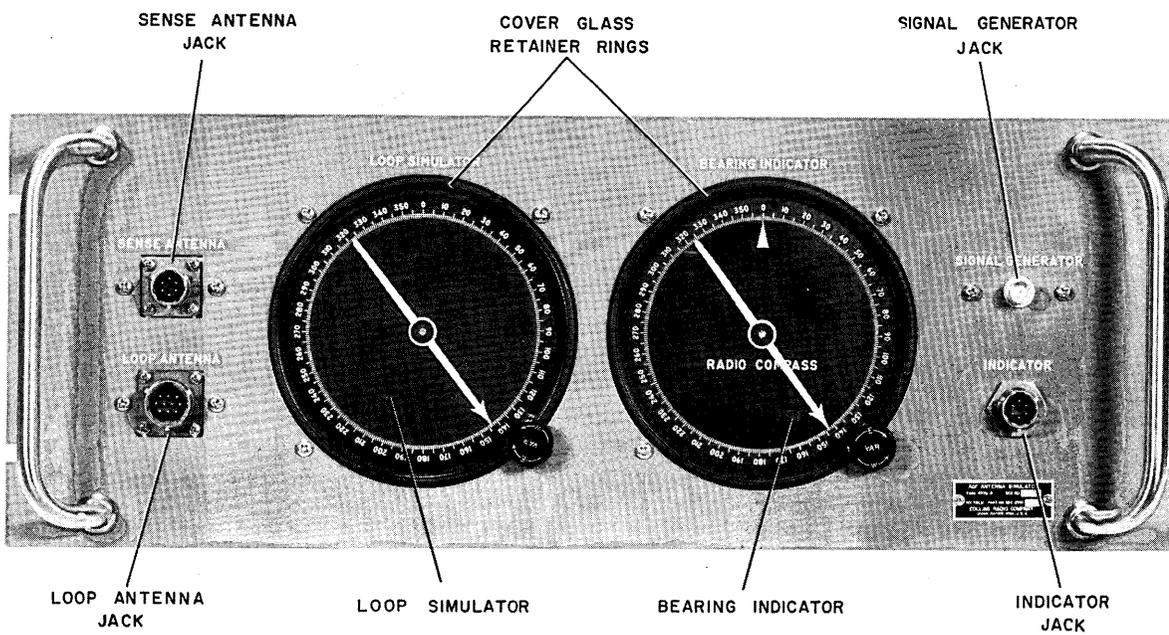
Figure 3-1. 477U-2 ADF Antenna Simulator, Front Panel
