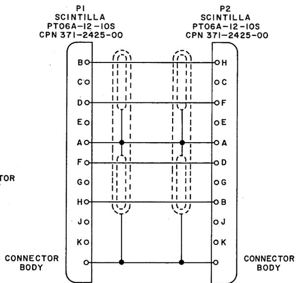
Figure 7-2. Simulator R-F Input Cable, Sense Cable, and Loop Cable, Schematic Diagram
