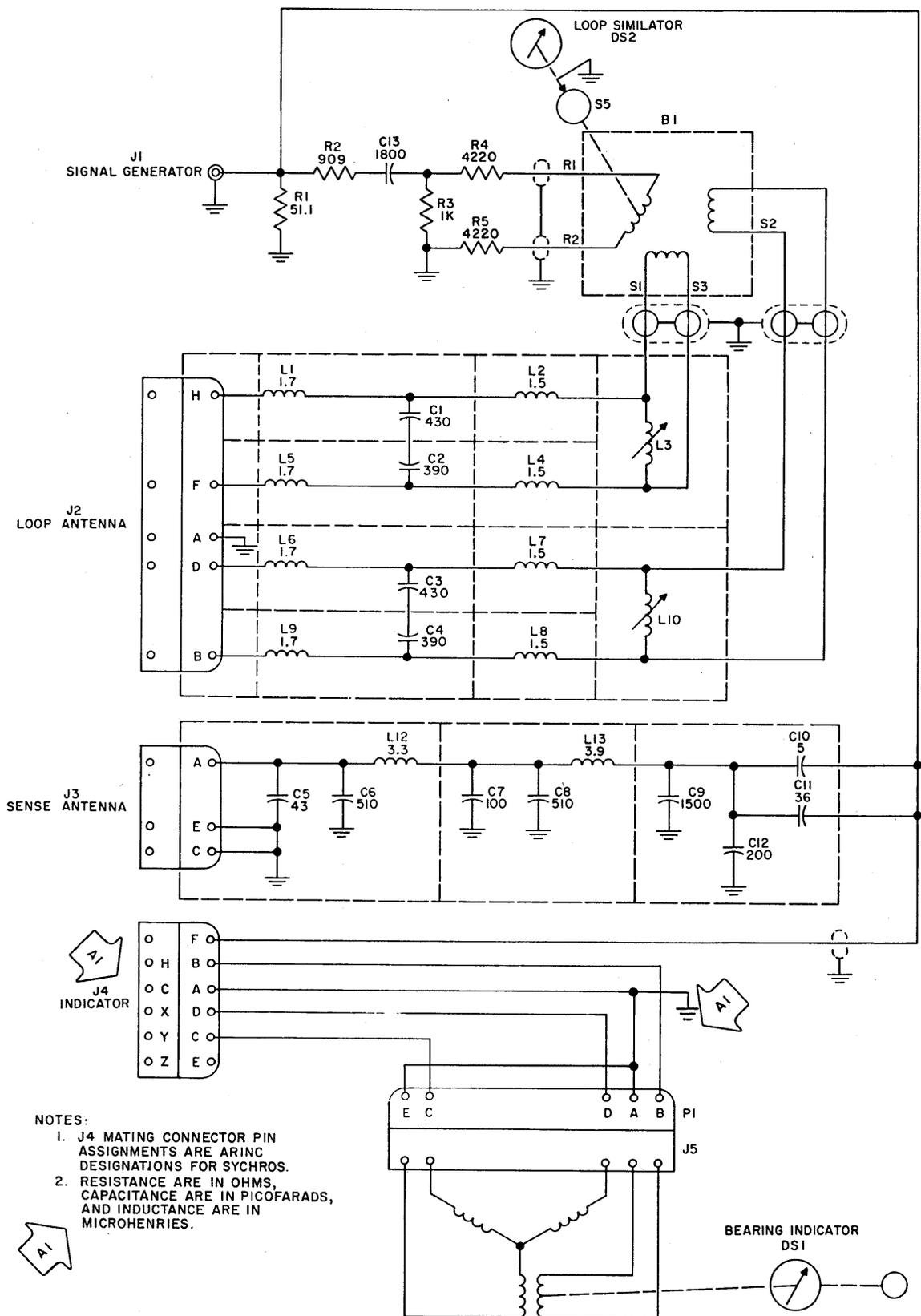
Figure 7-1. 477U-2 ADF Antenna Simulator, Schematic Diagram
