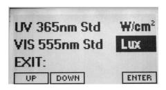
Press ENTER to return to left column, DOWN to highlight EXIT and ENTER again to access UNITS.
