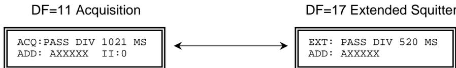
The detection time of each DF=11 and/or DF=17 message will be displayed. If the time interval is between 0.8-1.2 sec. - "PASS" is displayed. If the time interval falls in the 1.6-2.4 sec. range - "DIV" (Diversity) is also displayed. The aircraft address is also shown.
