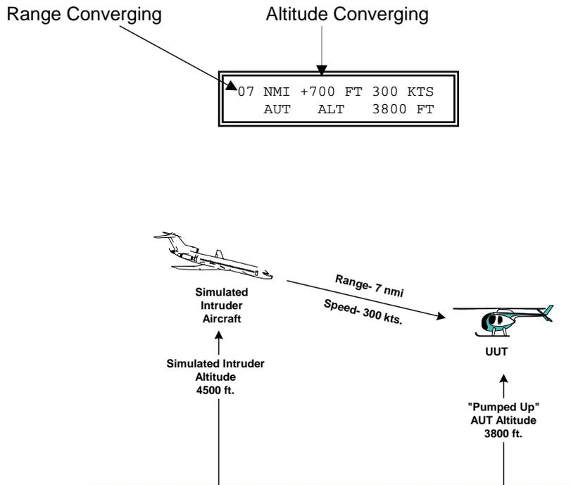
Once the Intruder Simulation reaches 0, the simulation will reverse direction and return back to 14 nmi.
