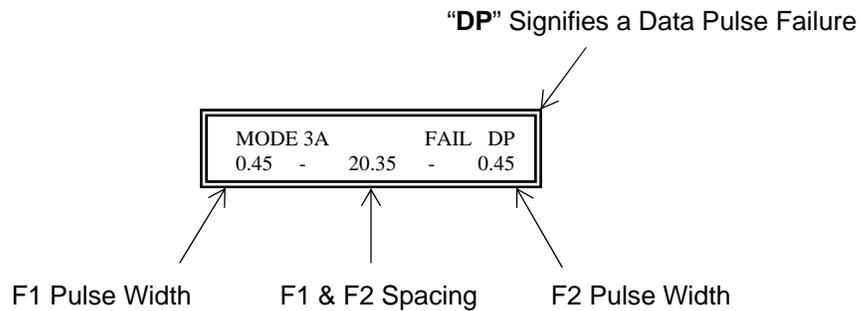
A “**FAIL**” signifies a F1/F2 Width failure, or a Framing Pulse Spacing Failure.
