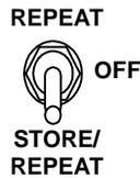
By placing the **STORE/REPEAT** switch to the “UP” position, the Test Set will continually retest the selected mode until the switch is returned to the “OFF” position.
