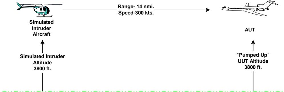
The Scenario will run from 14 nmi. to 0 nmi. and return back to 14 nmi. It will continue this cycle until another scenario is selected, the Test Set is turned "OFF" or times out.
