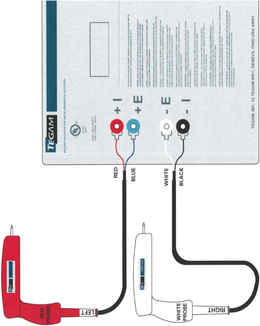
Figure 2a: HTP-101A Probe Connections
