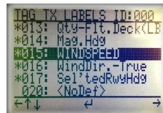
Fields that can be edited within a selected label are the data, SSM and SDI fields. The Parity is automatically created from the entered value and will be set to ODD. However, it is possible to edit the Parity value by writing to Bit-32 directly. Navigation of the screen is by use of the arrow keys.
