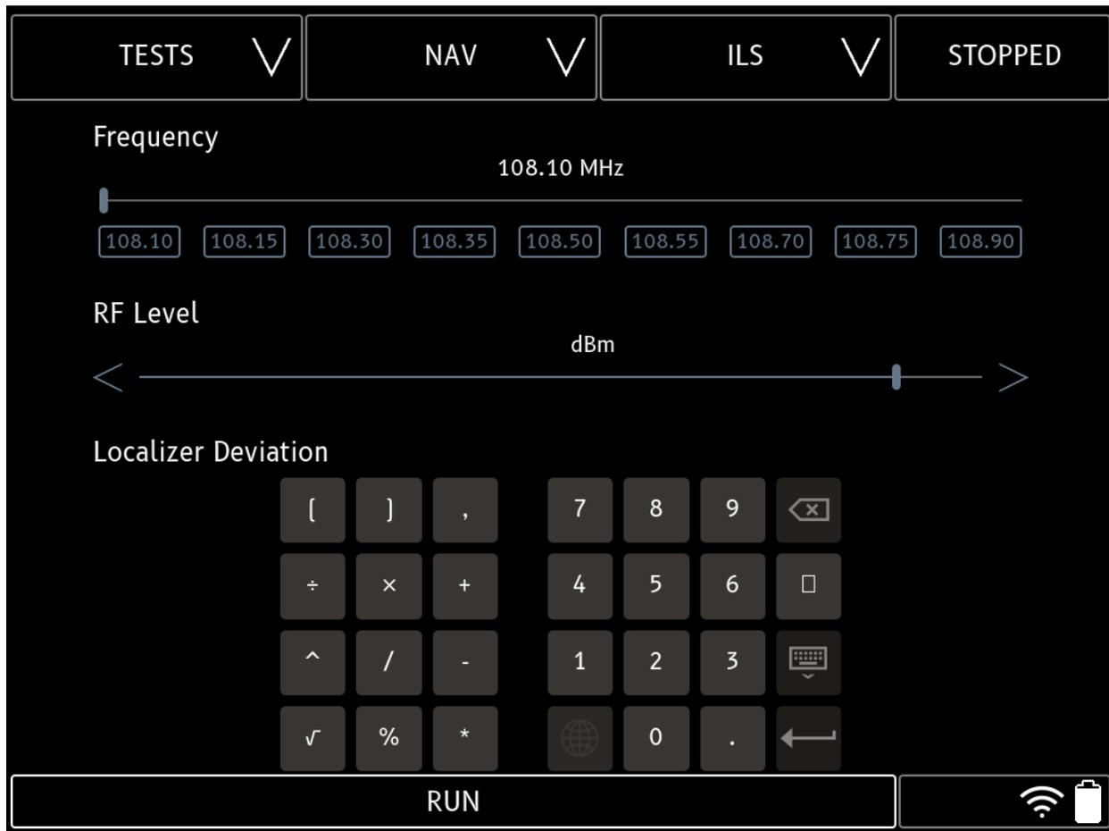
All sliders can be moved directly using the touchscreen, or by entering via an on screen numeric keyboard by touching the control value. For RF levels, enter as negative values (for example -15). Text fields will raise an alphanumeric keyboard.
