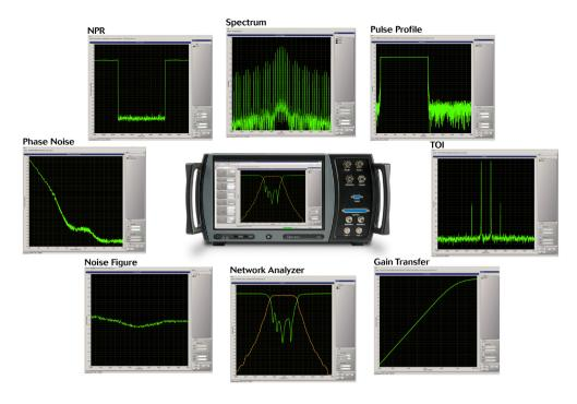
Figure 1. The 7700 includes a complete measurement suite that would normally require a full rack of instrumentation.
